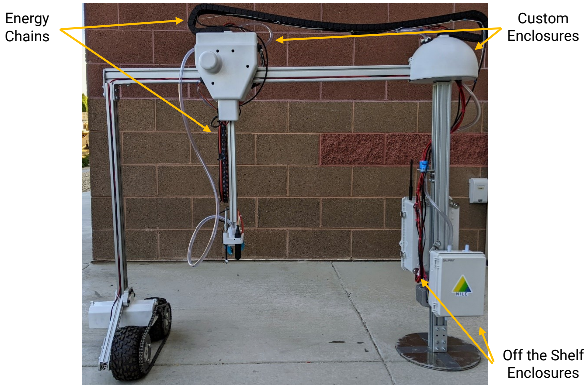
Figure 6. Cable Management Overview
