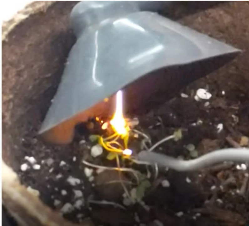
Figure 38. HVEC eliminating an undesired plant
