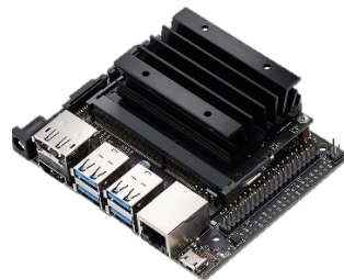
Figure 27. NVIDIA Jetson Nano
