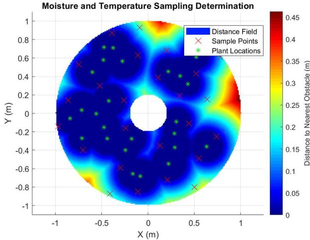
Figure 7. Distance-based soil sampling algorithm
