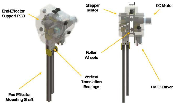
Figure 2. Trolley mechanical design
